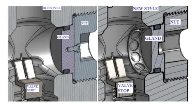
600, 1000, 1300 bhp pump fluid ends for 2.75" and 3.00" plungers:
