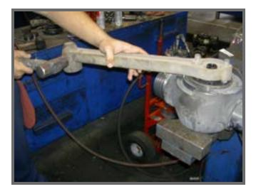
• Hit valve wrench with hammer a couple times to make sure it is firmly seated. This is necessary to fully compress the plug seal o-ring.
