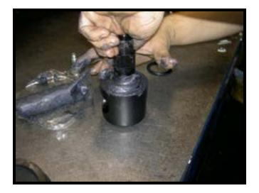
• Apply a thin film of valve grease to the entire O.D. of the **plug (10) [9]**.
