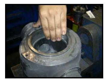
• Check the **pins (14) [10]** in the bottom of the valve body pocket to make sure they are not bent or broken.
