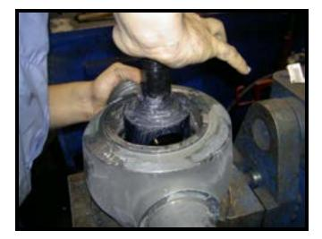
• Apply anti-seize compound to the threads on the valve body and **body cap (5) [16]**, along with a light coat of valve grease on the body cap sealing surfaces.
