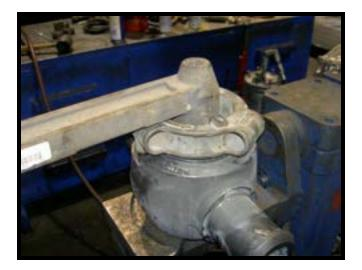
• Apply anti-seize compound to the threads on the SafeTap<sup>™</sup> grease fitting (1) [18].
