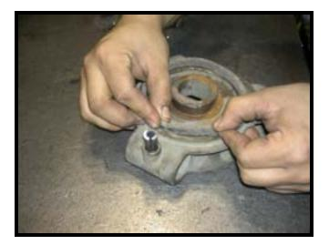
Install the handle adapter (3) [3] onto the top of the plug (10) [9].
