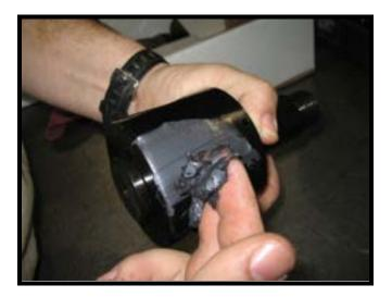
Push the assembled plug with seals into the valve body, making sure it is properly aligned with the segment set (12) [12] and side segments (11) [11] until it is seated all the way down. Make sure the valve is in the open position.
