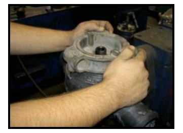
Secure the handle adapter (3)[3] with handle lock-nut (2) for 1" & 2" TE valves or hex-hd cap screw [1] and flat washer [2] for 3" TES valves.
