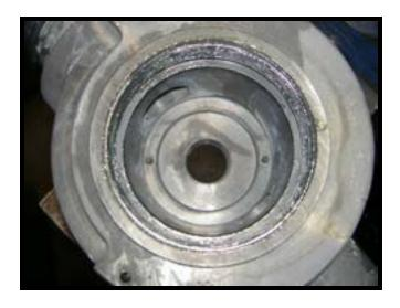
• Lightly lubricate the threads with anti-seize, then screw the clean **body cap (5) [16]** all the way into the valve body to make sure the threads are not damaged.
