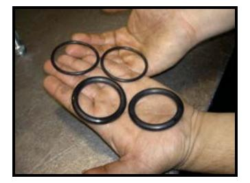
• Coat the o-rings (13) [13] with valve grease and install onto the segment set (12) [12].
