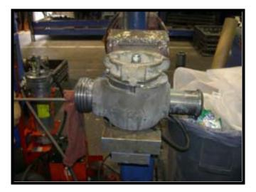
• Ensure that the plug, segment set, and valve bore are properly aligned.
