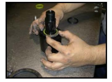
• Apply valve grease to both seals.
