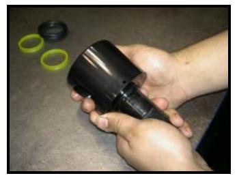
Install the upper and lower plug seal rings (8) [7] and o-rings (9) [8] onto the ends of the plug (10) [9].
