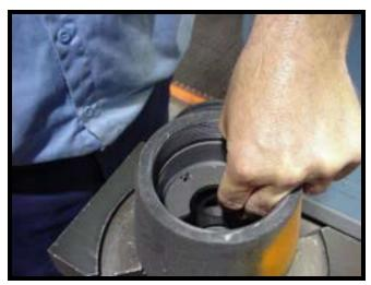
Apply a thin film of lubricant to the recess in the valve body (8) and install the plug seal (9) with the groove facing out.
