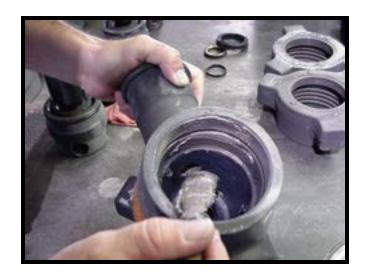
o Install the plug (10), inserts (12) and adjusting nut (14) assembly into the valve body. Keep in mind that the roll pins must line up with the groove on the Inserts.
