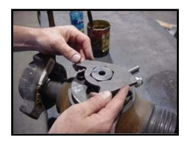
o Install the **handle adapter (4)**. Align the plug arrows with the handle adapter tabs.
