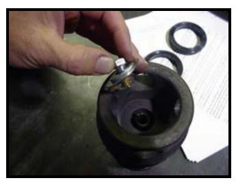
o Apply thread anti-seize to the adjusting nut threads in the valve body or on the adjusting nut. It is not necessary to apply to both.
