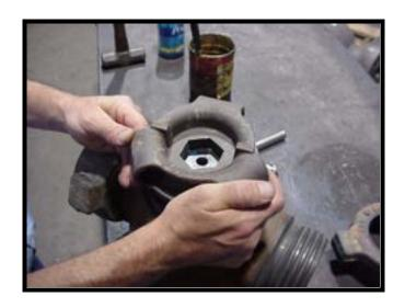
o Secure handle adapter (4) with the plug screw (1) and washers (2 & 3).
