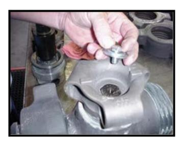
Inspect plug alignment and adjust as necessary with adjusting nut (14). Do not over tighten as this will cause excessive operating torque.
