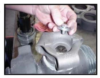
Inspect plug alignment and adjust as necessary with adjusting nut (14)
