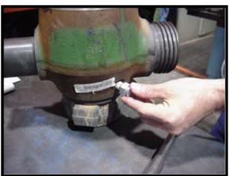
o Grease valve to a minimum of 3,000 psig in the open position. After greasing, actuate to burp valve. Repeat the following step.
