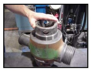
Apply thread anti-seize to the threads on the SafeTap™ grease fitting (7).
