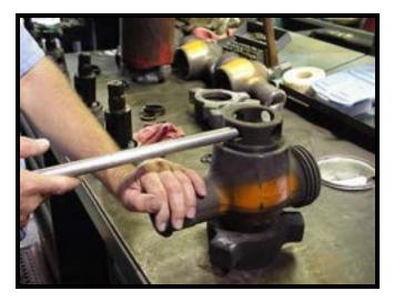
Apply thread anti-seize to the threads on the SafeTap<sup>™</sup> grease fitting (7). Install grease fitting and torque to 125 ft-lbs.
