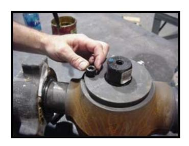
o Install **stop collar (5)**. Ensure that the stenciled side of the stop collar is facing up.
