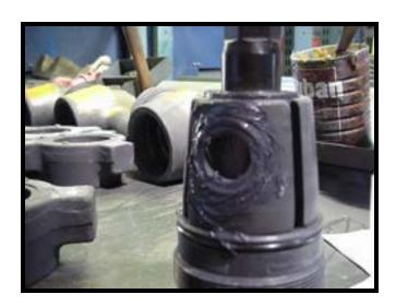
Apply thread anti-seize on plug screw. Secure the plug to the adjusting nut with the plug screw (1) and washers (2 & 3).
