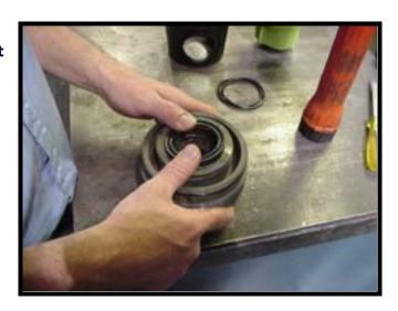
o Check the **plug (10)** outside diameter for surface defects such as scratches, dings, nicks, or sharp edges that could affect the sealing area. See
