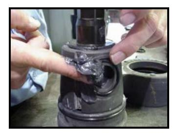
o Make sure the entire sealing surface is thoroughly greased.
