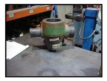
o Install the plug (10), UNIsert™ (12) and adjusting nut (14) assembly into the valve body. Keep in mind that the roll pins must line up with the groove on the Inserts.
