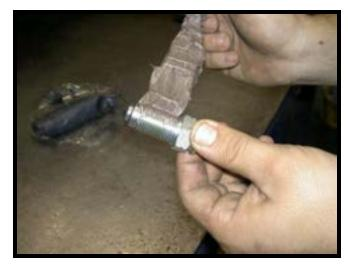
o Install SafeTap™ **grease fitting (7)** and torque to 125 ft-lbs.
