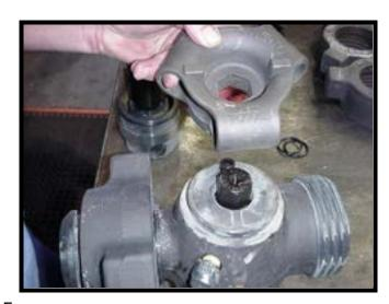
Secure handle adapter (4) with the plug screw (1) and washers (2 & 3). Apply thread anti-seize onto plug screw prior to installing.
