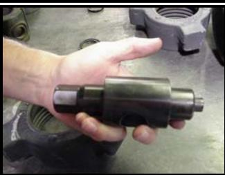
Apply grease to the plug seal
