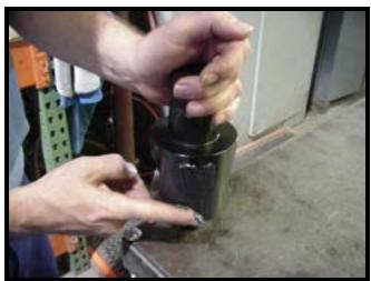
o Install the lower end of the plug (10) (opposite the hex) in the UNIsert™ (12) and adjusting nut (14) and push down until the plug shoulders on the adjusting nut.
