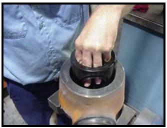
Apply a thin film of lubricant to the recess in the valve body
