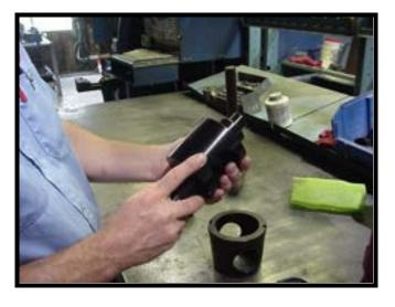
o Check the surface finish of the **UNIsert™** (12) making sure it does not have any scratches, dings, nicks or sharp edges that could also affect the sealing area. See <u>6.2 SANDING TIPS</u> for repair.
