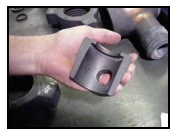
o Apply a thin film of grease to either the entire O.D. of the **plug (10)** or **inserts.** Do not apply grease to both parts.
