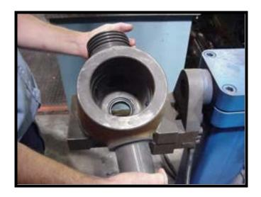
Apply a thin film of lubricant to the recess in the adjusting nut
