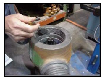
o Support the valve so that the **plug (10)** hex can pass through unobstructed.
