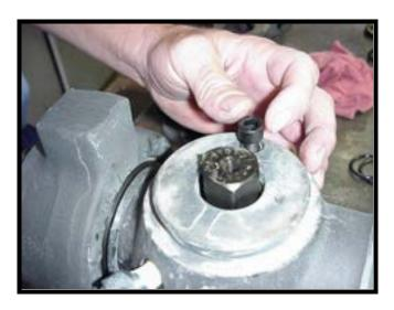
o Install **stop collar (5)** and **handle adapter (4)**. Ensure that the
