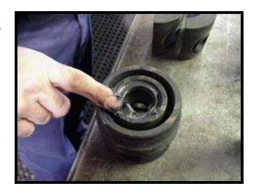
o Install the lower end of the plug (10) (opposite the hex) in the adjusting nut (14) and push down until the plug shoulders on the adjusting nut.
