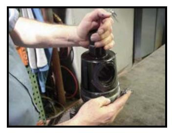
o Secure the plug (10) to the adjusting nut (14) with the plug screw (1) and two washers (2 & 3). Apply thread anti-seize onto the plug screw prior to installation.
