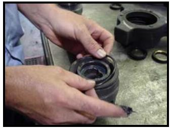
Check the roll pins (15 & 16) in the valve body by gently sliding a set of inserts (12) into the valve. The inserts (12) should move freely up and down the length of the roll pin slots without interference.
