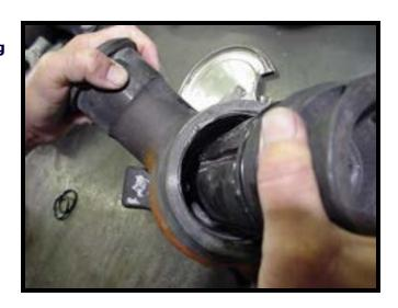
Support the valve so that the **plug (10)** hex can pass through unobstructed.
