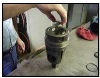
Apply thread anti-seize to the adjusting nut threads in the valve body or on the adjusting nut. It is not necessary to apply to both.
