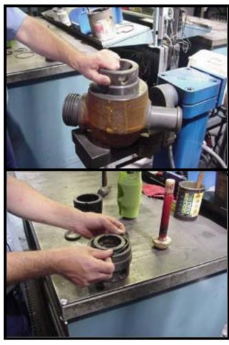
o Check the roll pins (15 & 16) in the valve body by gently sliding a UNIsert™ (12) into the valve. The UNIsert™ (12) should move freely up and down the length of the roll pin slots without interference.
