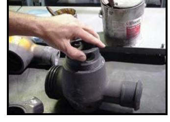
After inspection, remove the adjusting nut (14), grease the sealing groove and install the adjusting nut o ring (13) in the groove.
