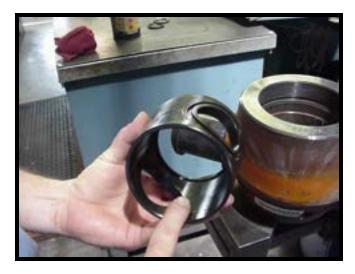
o Inspect the **adjusting nut o-ring (13)** for any possible non-conformity.
