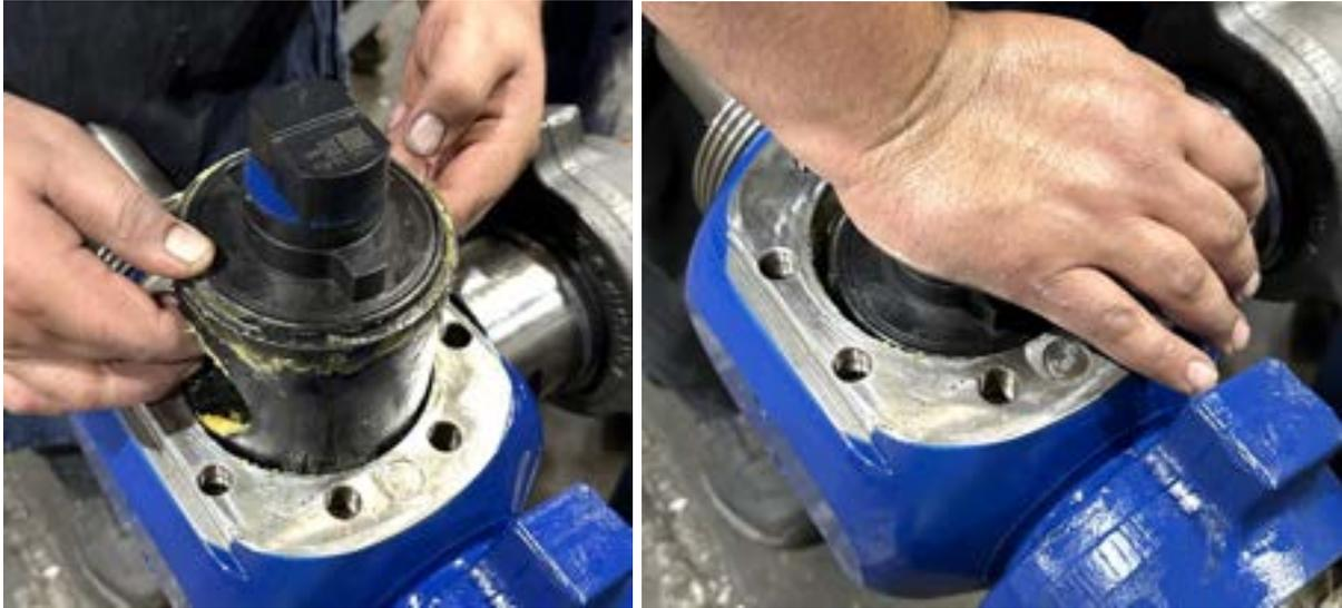
11. Rotate the plug to the open position and remove the seat tools (if used).
