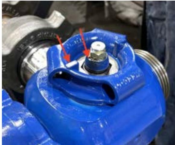
20. Replace the washer then snap ring. A plastic tool is provided in repair kits to push the snap ring down and into the groove.
