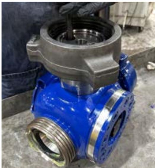
4. Lift the valve using LSA0003 lift sub and attach to the work table with the STA0008 adapter.
