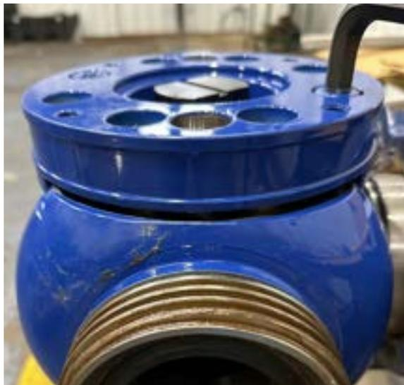
17. Once the cap is fully seated against the valve body, install the remaining 6 screws and tighten with hex key until fully engaged. Then use a torque wrench set to 230 ft-lbs to tighten all 8 screws in a cross pattern.
