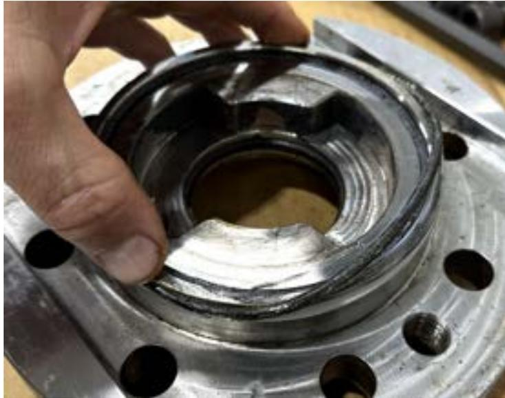
13. Place the cap on the valve such that the screw holes and keys are aligned with those on the valve body. It does not matter which direction the cap goes on otherwise.
