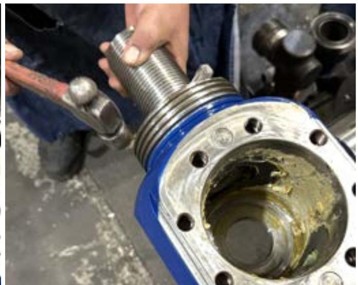
6. Apply a light coat of plug valve grease onto the plug stem seals then snap them onto the backup rings.
