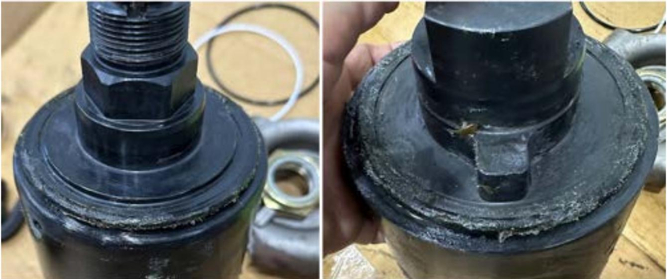
8. Before continuing to the next step verify rotational alignment on both seats. If adjustment is needed, loosen the seat tool wingnut and make the necessary adjustment, then retighten the wingnut.
