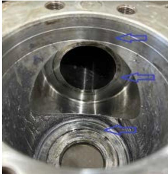
2. Apply a small amount of grease to the seat seals then insert into the groove of each seat.
