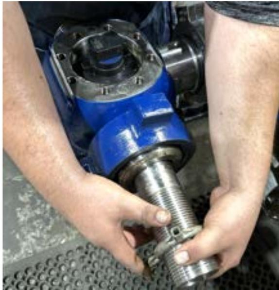
12. Place the seal backup ring onto the cap and push to the bottom of the groove. One side of the backup ring is cupped and should face the seal, but installing it in either direction is acceptable. Apply a light coat of plug valve grease on the cap seal then place it into the groove on top of the backup ring. Go around the seal with your finger to evenly distribute it in the groove.
