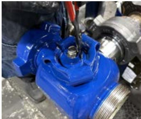
6. Once the snap ring, washer, and handle have been removed, loosen the STA0008 wingnut and rotate the valve so that the cap is facing up. Retighten the wingnut.
