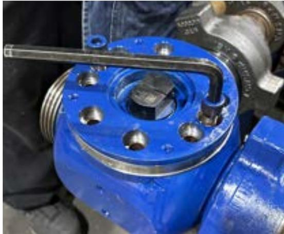
10. Set the cap aside then remove the seal and backup ring with a pick and discard them.
