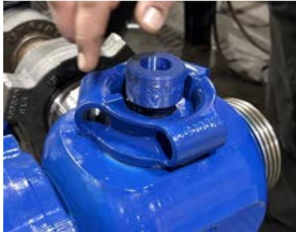
21. Rotate the plug to full open and full close a few times to verify movement is smooth and there is no binding or roughness. If the rotation is not smooth, disassemble the valve and inspect for foreign materials.
