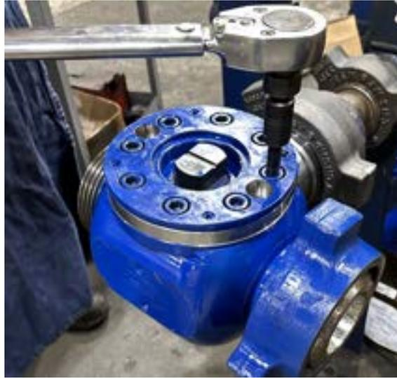
18. Reinstall the plastic plugs into the jack screw holes.
