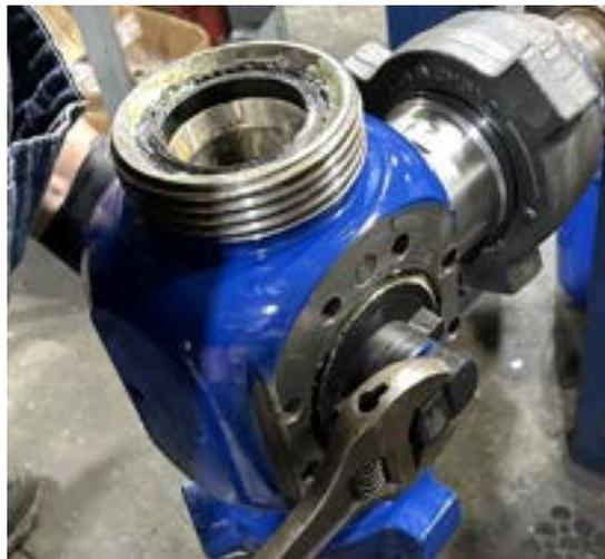
12. Once the plug has been pushed partially out, grasp it using the bore and pull straight out in one continuous motion.
