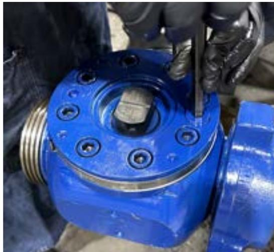
8. Next remove all 8 screws using the 1/2" hex key and breakover bar.
