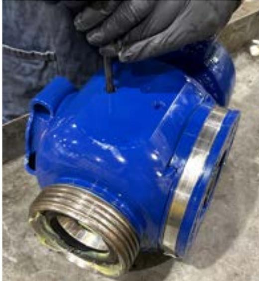
3. Attach STA0008 service tool to the side of the valve using a 1/2" hex wrench.
