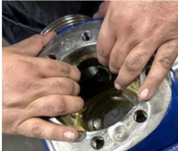
5. The seat tool may be used to ease plug installation but it is not mandatory for assembly, the plug may be pressed directly through the seats.
