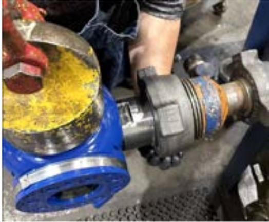
5. Rotate valve so that the handle is facing up and tighten the STA0008 wingnut to prevent rotation. Use snap ring pliers to remove the snap ring holding the handle to the plug.
