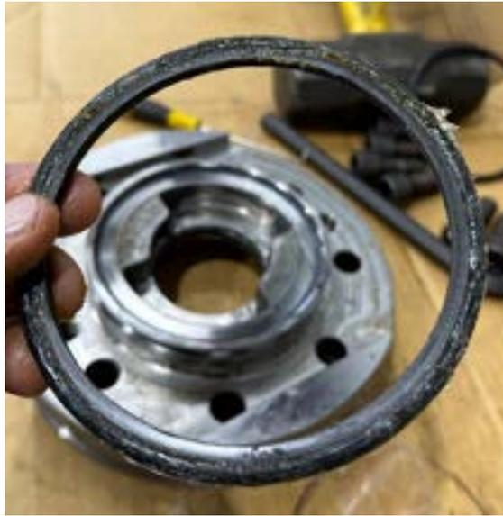
7. Press the seals onto each end of the plug being sure they are firmly seated. There should be enough grease present to keep the bottom seal from falling off.
