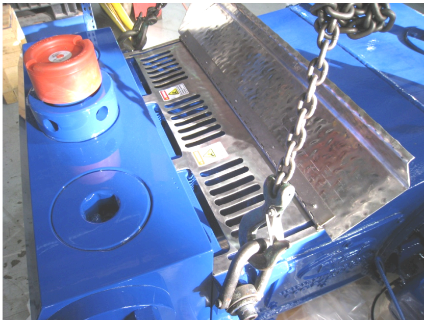
PLUNGER PORT SAFETY GUARD AND WEATHER SHIELD
